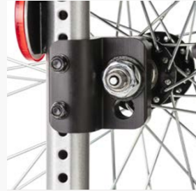
Wheelbase extension by turning the varioblock backwards
