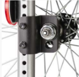
Wheelbase extension by turning the varioblock backwards
