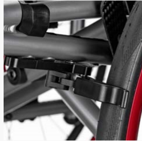
Innovative light brake, swivelling, aluminium
